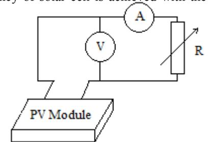
**1.10 Photovoltaic Array:** A typical silicon cell can produce upto 0.6 V and upto 6 Amp i.e. equivalent to about 3 W power. The cell size varies from 1 cm to about 10 cm across. To increase power output, cells are electrically connected in series and parallel to absorb as much light as possible to produce desired voltages and current. A number of cells are combined to form a **Module**. When modules are combined we get a Panel. Panels are combined to get an **array**.
