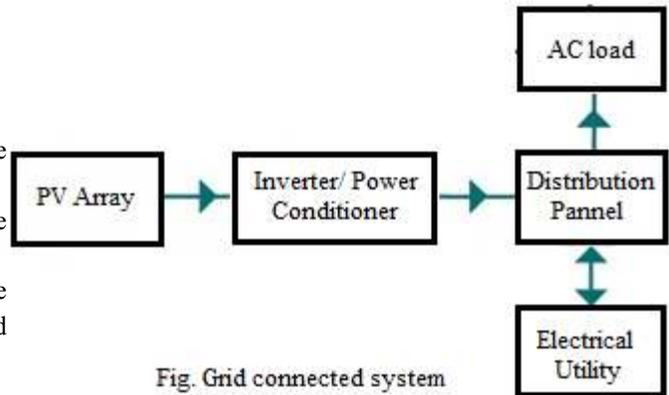
Fig. Grid connected system
