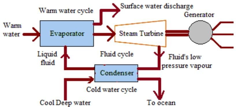
Fig.5. Closed or Anderson Cycle OTEC System
