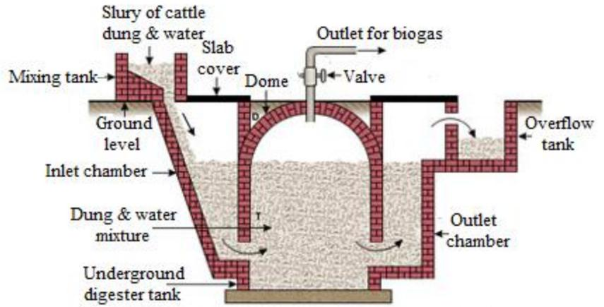
Fig.2. Fixed dome type biogas plant (Janata Model)
