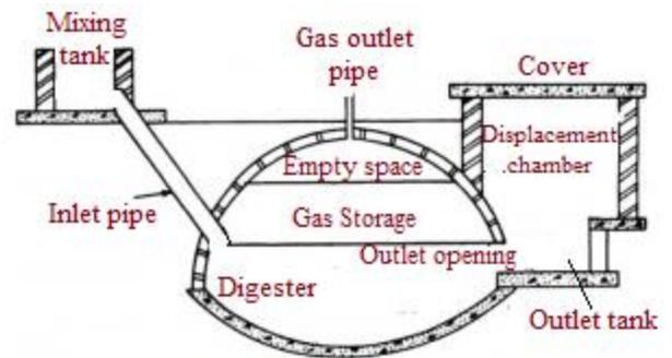
Fig.3. Deenbandhu biogas plant
