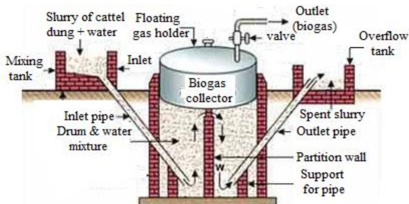
Fig.1. Floating Drum type biogas plant (KVIC Model)
