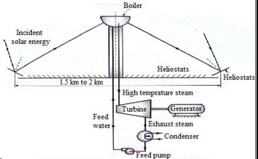
Fig. Central tower receiver power plant using heliostats
