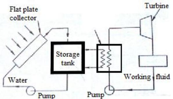
Fig. Working of low temprature solar power plant
