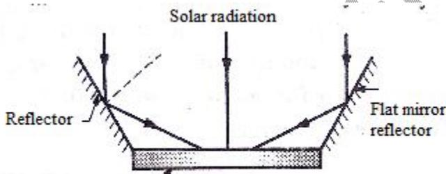
Fig. Flat Plate collector with plane mirror reflector
