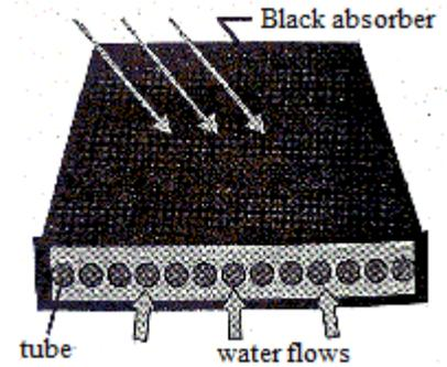
**2.5.2 Construction and Materials for Flat Plate Collectors:**
