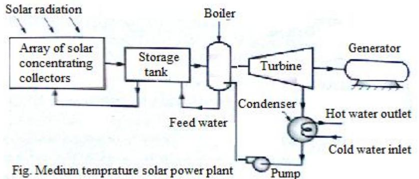
Fig. Medium temprature solar power plant
